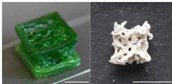
Fig. 1: Left: AM fabricated biotic scaffold with PCC 7002. Right: 30 days incubated biotic scaffold after thermal decomposition. Scale bar: 1 cm.
