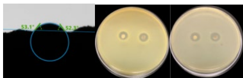
Fig. 2(a): Sponge hydrophilicity; (b) Antibacterial activity against gram-positive and gram-negative bacteria respectively.
