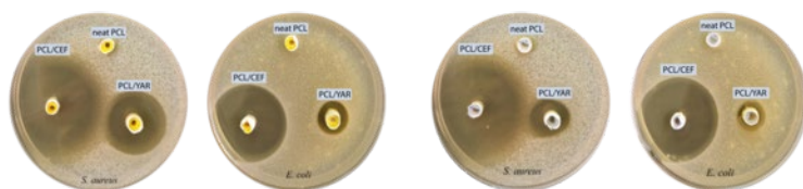
Figure 1. Inhibition zone diameter of nanofiber mat coatings onto rubber and silicone urinary catheters against S. aureus and E. coli
